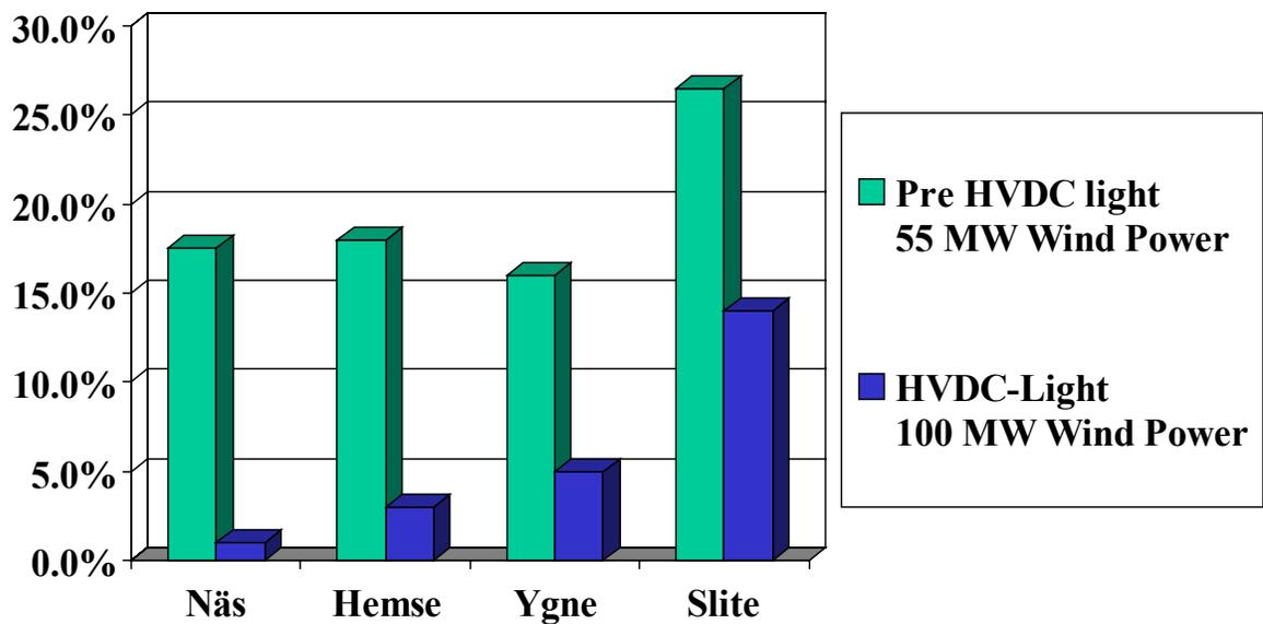
**Figure 3.** *Voltage drop during obtained previous and after HVDC-Light connection during a short circuit in the AC network.*
