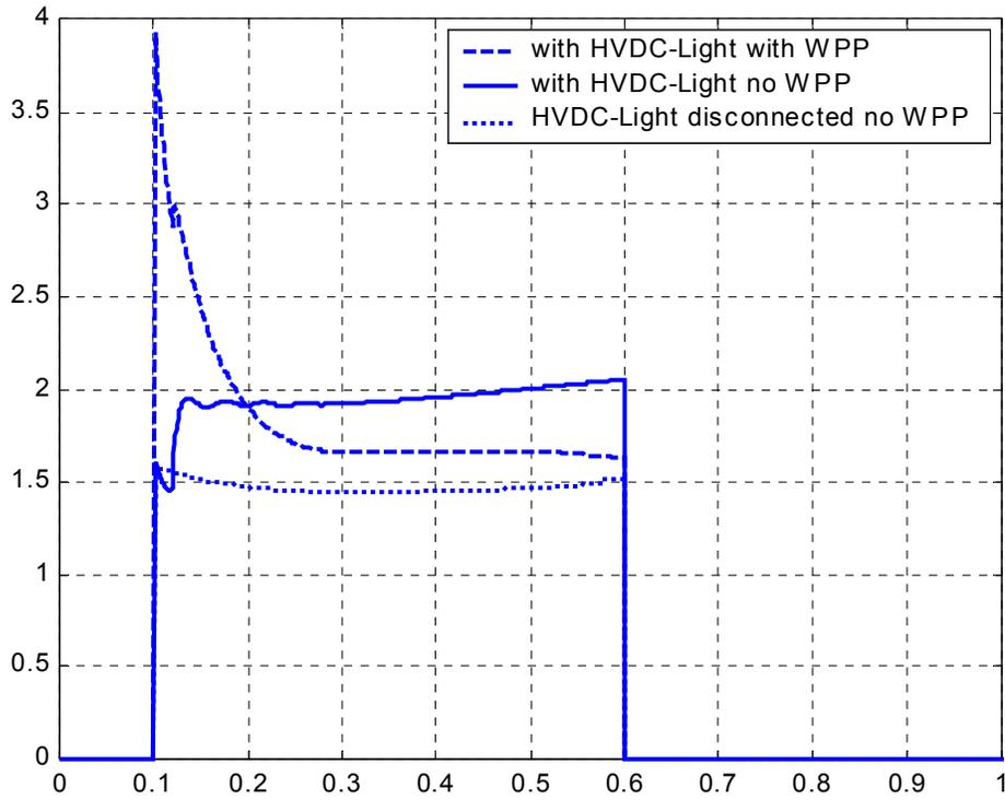
**FIGURE 4. EFFECT OF HVDC-LIGHT AND WPP ON THE FAULT CURRENT DURING SHORT CIRCUIT AT NÄS**
