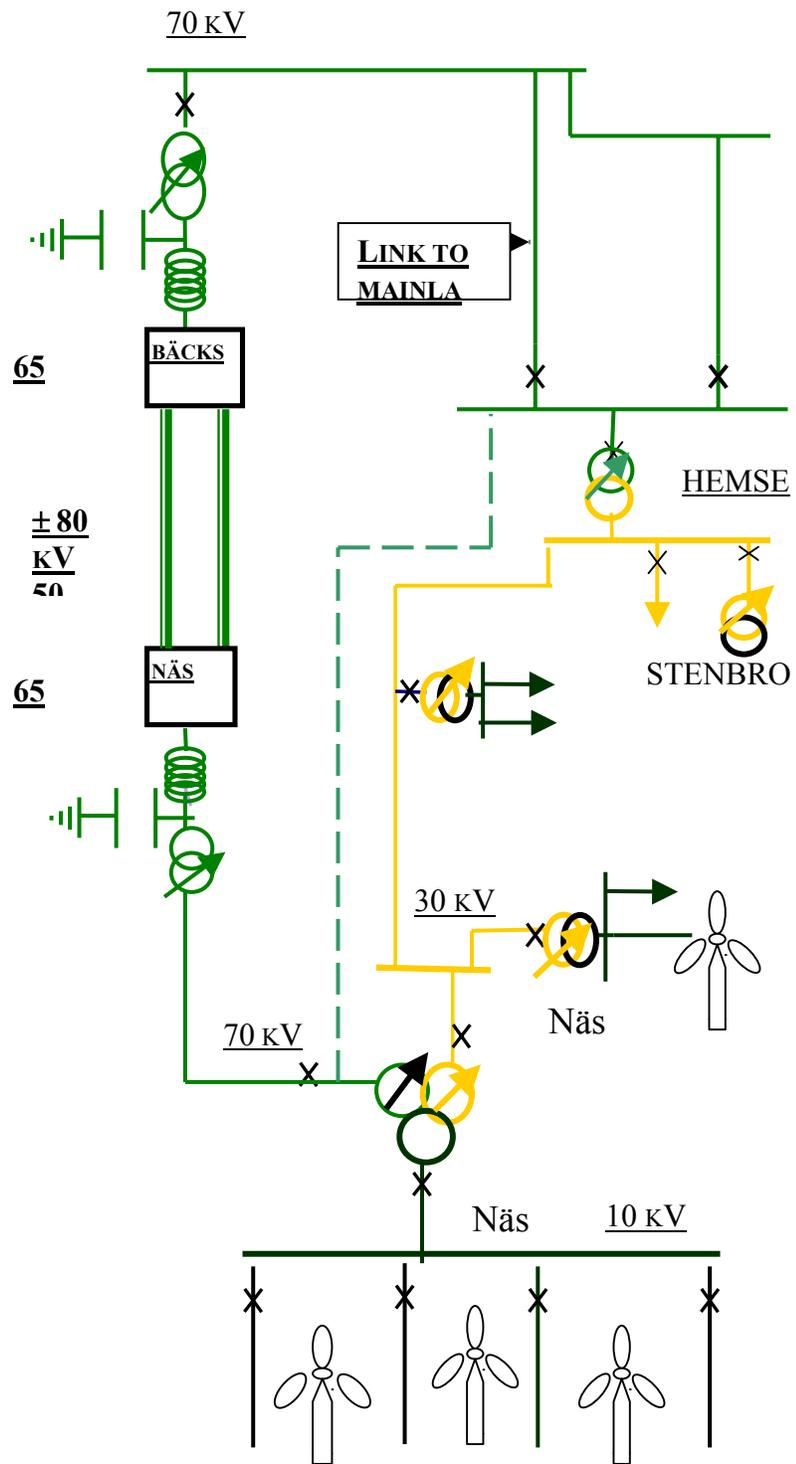
**FIGURE 1. SIMPLIFIED SCHEME OF THE AC NETWORK WITH HVDC-LIGHT CONNECTION**
